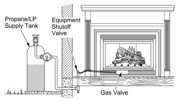
Figure 34 - Checking Gas Joints for Propane/LP Gas Fireplace
